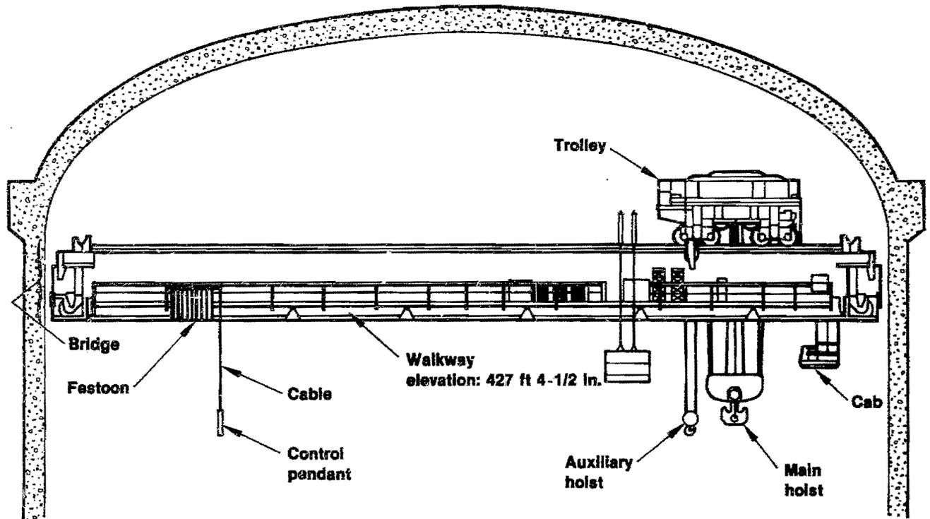
Following nearly a year of inspections, analyses, repairs, replacements, and no-load operational testing, the polar crane at TMI-2 is structurally, mechanically, and electrically ready to undergo load testing—the final stage in preparation for reactor vessel head lift operations. The 500-ton Whiting polar crane installed in the TMI-2 Reactor Building became inoperable as a result of the March 1979 accident. Figure 9 shows the main components.
