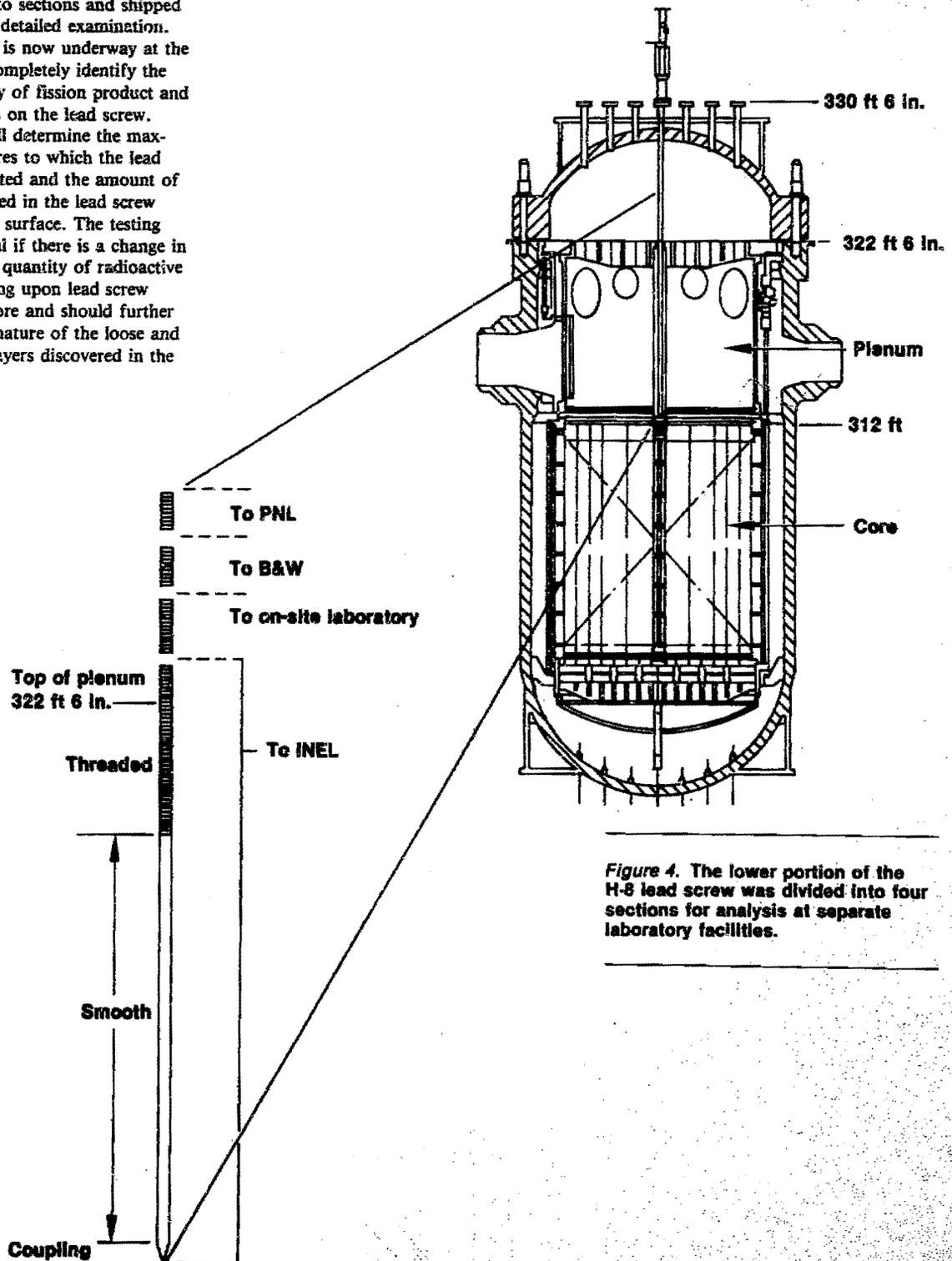
Figure 4. The lower portion of the H-8 lead screw was divided into four sections for analysis at separate laboratory facilities.
