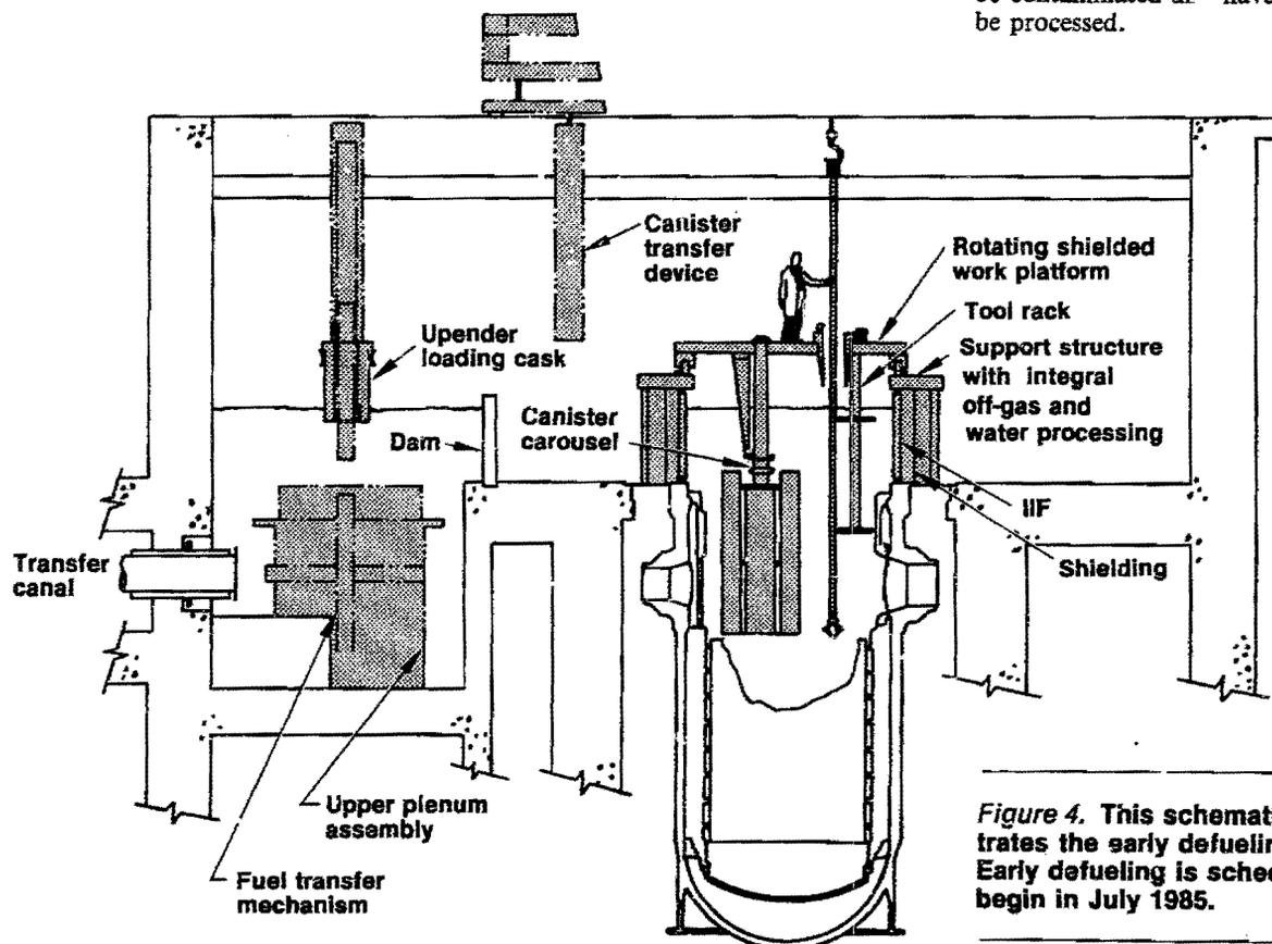
**Figure 4.** This schematic illustrates the early defueling system. Early defueling is scheduled to begin in July 1985.
