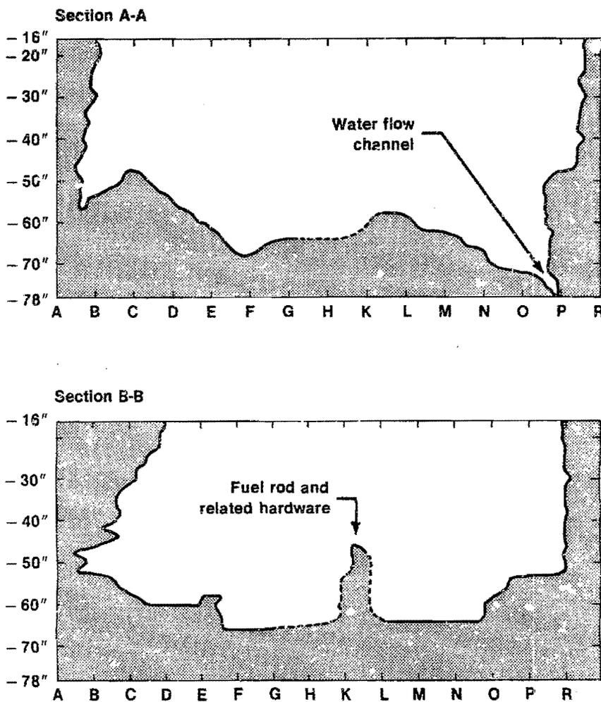
Using the data collected from the sonic sensing head, engineers also were able to plot cross sections of the void. Two such cross sections are presented in *Figure 15*. The solid lines in these drawings were produced from actual data, while the dashed lines are approximate locations obtained by extrapolation or interpolation. (A few areas of the rubble bed were not within the range of the acoustic transducers.)
