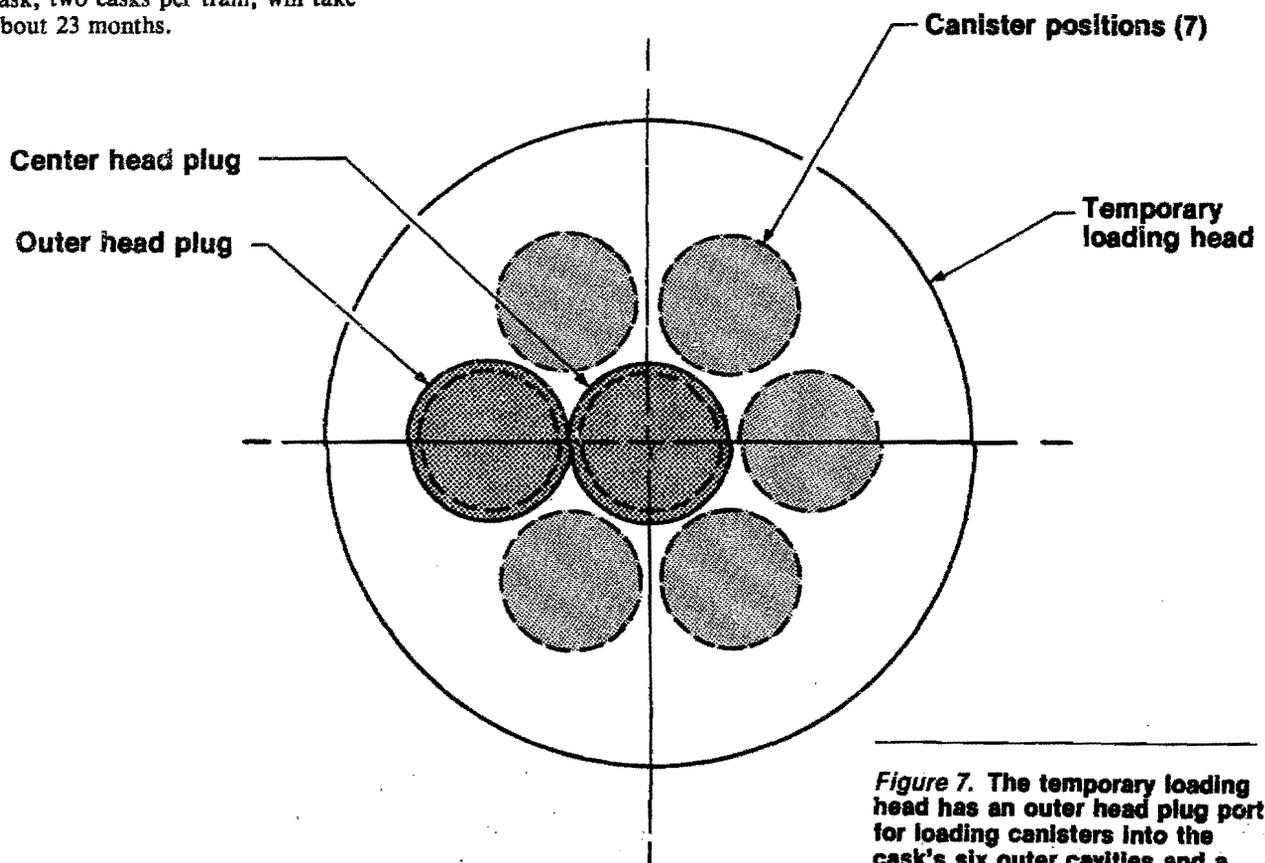
**Figure 7.** The temporary loading head has an outer head plug port for loading canisters into the cask's six outer cavities and a center head plug port to load the seventh canister into the center cavity.
