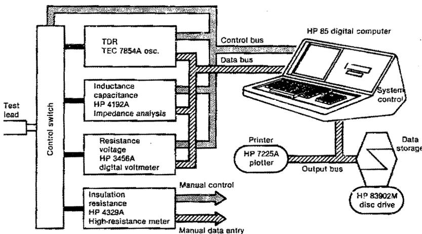
Figure 1. Electrical circuit characterization and diagnostic system.
