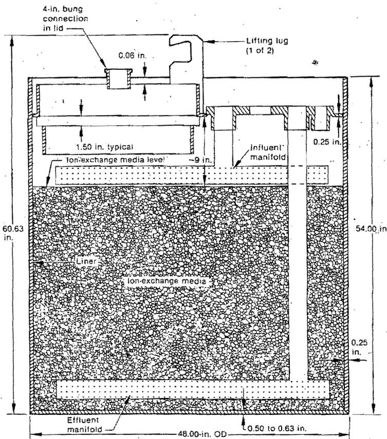
*Figure 14* Cutaway sketch of EPICOR II prefilter liner.
