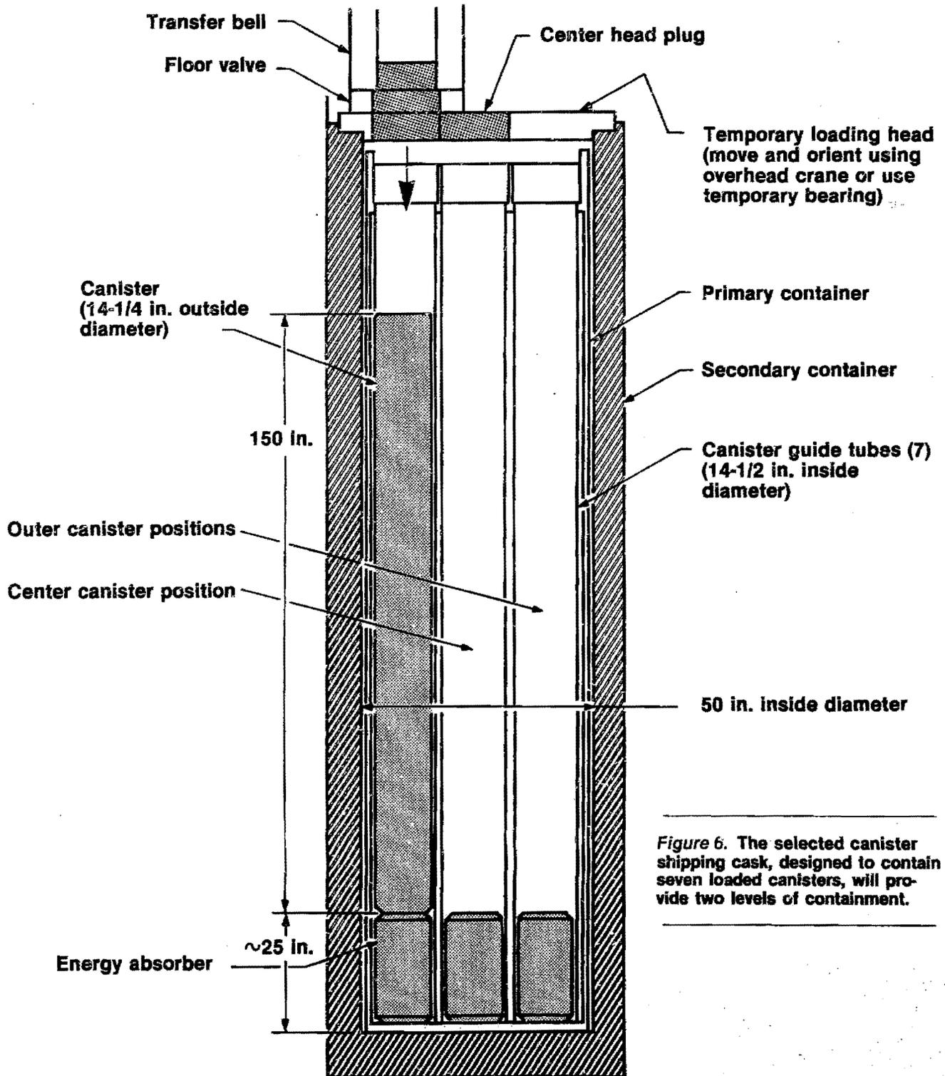
Figure 6. The selected canister shipping cask, designed to contain seven loaded canisters, will provide two levels of containment.
