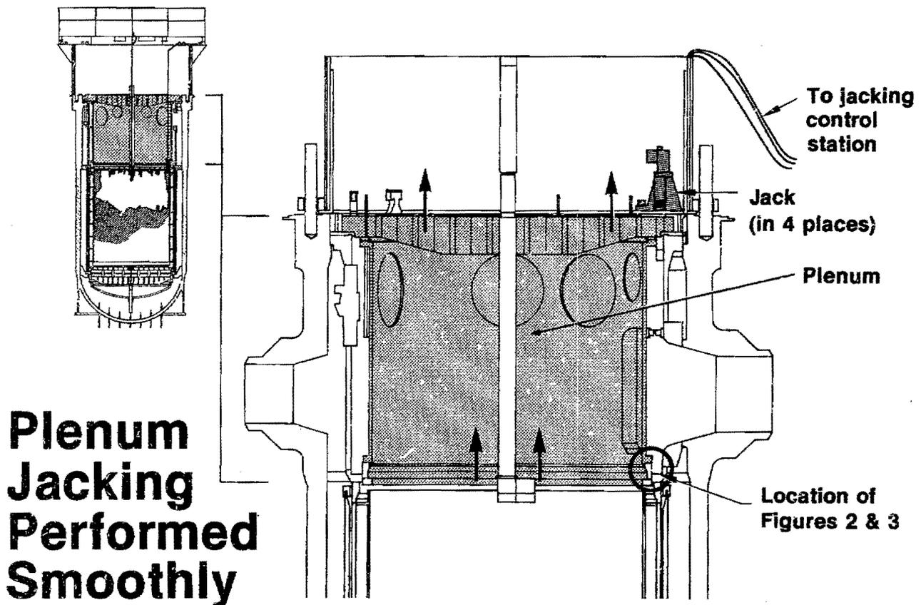
The plenum assembly, the 55-ton cylinder on top of the core containing the guide tubes for the control rods, was jacked in December 1984 in preparation for its removal in May (see Figure 1). Removal of the plenum will provide access for defueling the damaged reactor.
