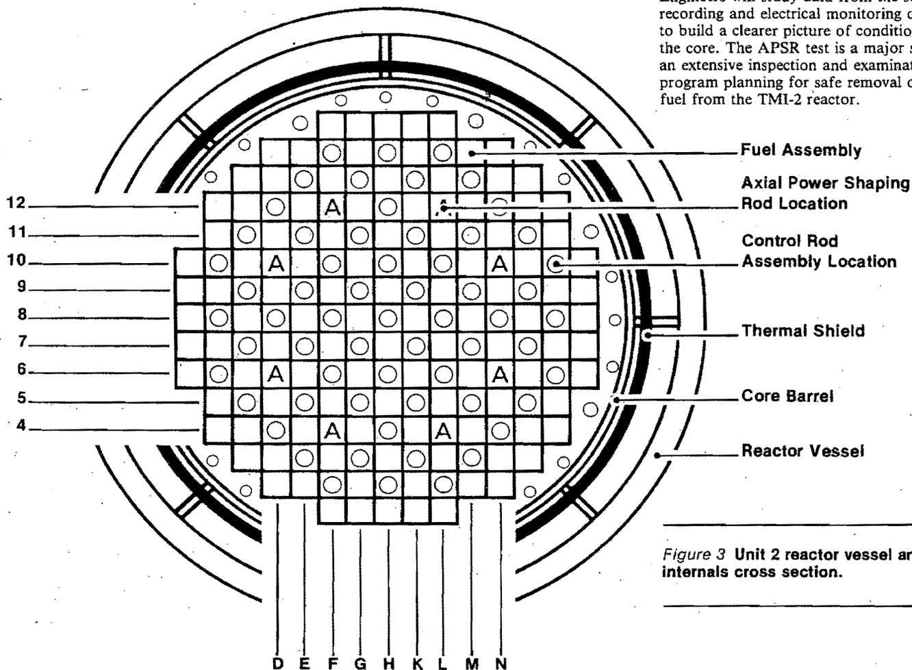
*Figure 3* Unit 2 reactor vessel and internals cross section.
