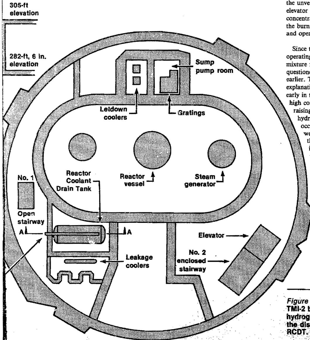
Figure 6 As this drawing of the TMI-2 basement indicates, the hydrogen was released through the discharge duct from the RCDT.
